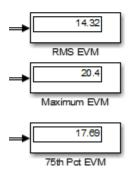
Change the **I/Q amplitude imbalance (dB)** value in the I/Q Imbalance block to 2 dB. You can see that the all the MER and EVM metrics degrade.
