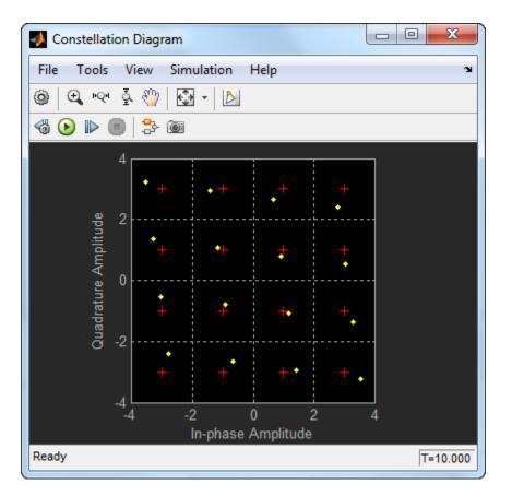
You can see that I/Q amplitude and phase imbalance has shifted the constellation diagram so that each symbol is not exactly equal to its reference symbol (shown in red). Change the I/Q Imbalance block to see the effects of differing imbalances on the constellation diagram.
