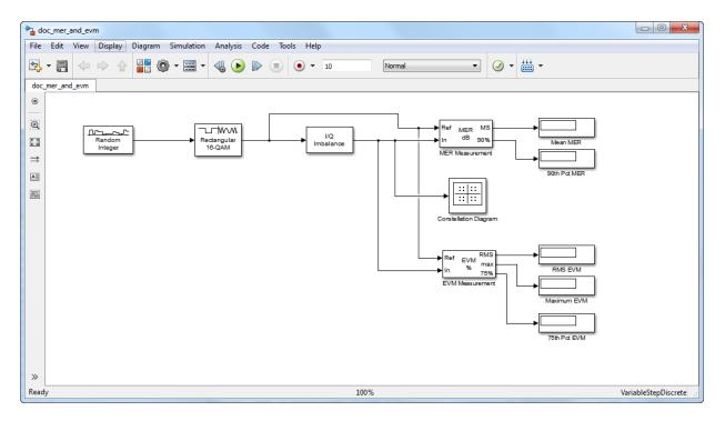
The I/Q Imbalance block is set to that the I/Q amplitude imbalance (dB) is set to 1 and the I/Q phase imbalance (deg) is set to 15.
